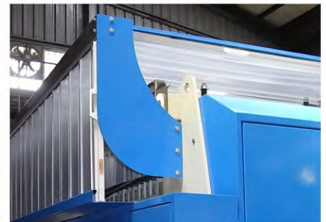
Removable protection-lens design
