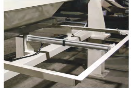
Cylinder motion type plate: Sludge falls directly, facilitates cleans up and takes away, the working environment is clean and neat.
