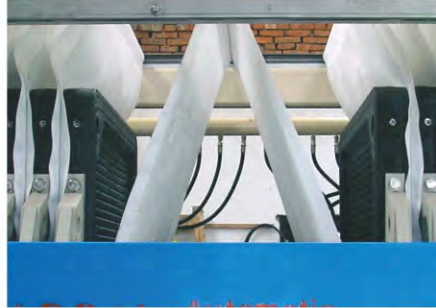
Auto Cake Discharge : Clothes shaking & shaped "A" to help cake dropping easily.
