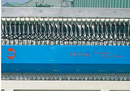
Auto Cloth Back - Washing System : Close, Backward washing cloth as well as feeding pipe in one time.
